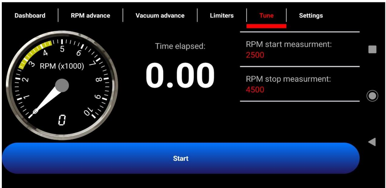
This allows you to measure the acceleration time between the 2 rpm settings.
